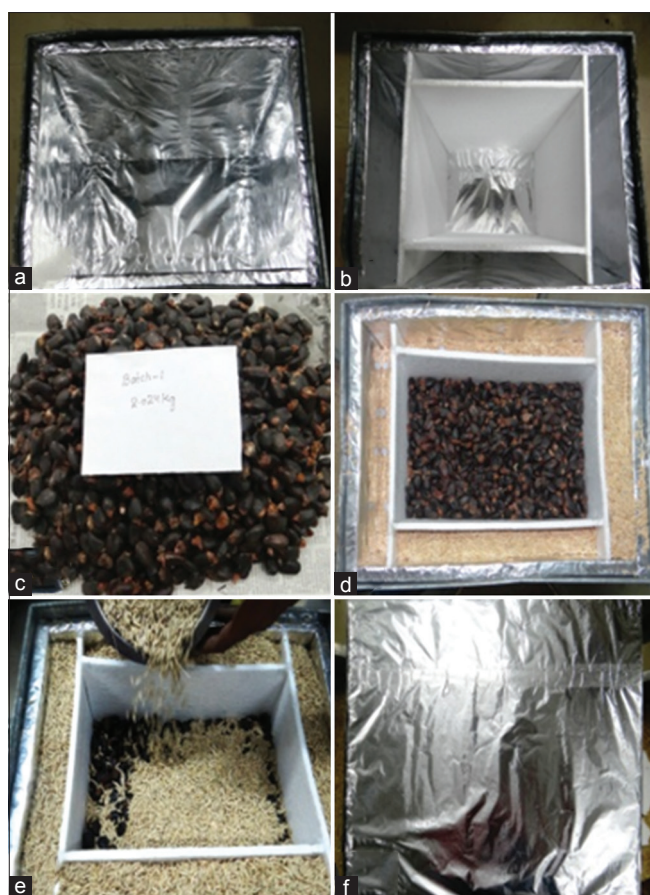
Figure 2: Curing experiment. (a) Aluminum box covered inside with wrapped thermocol, (b) box with another cabin prepared from plane thermocol sheets, (c) fresh Bhallataka batch before curing, (d) Bhallataka filled in-between Barley fruits, (e) completion of the process of preservation, (f) closed box for 4 months
