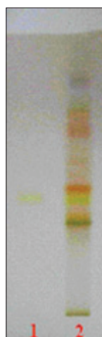
Figure 3: Detection of piperine from Piper longum and Eladi Gutika at 550 nm using HPTLC, track 1 – Piperine standard, track 2 – Eladi Gutika
