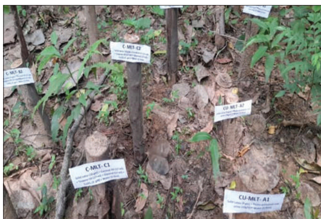
Photoplate 2: Showing solid wood sticks experiment set up
