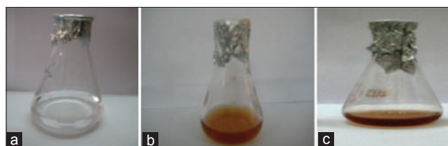
Figure 2: (a-c) Color change during phytoreduction from silver nitrate to silver nanoparticles over for Ailanthus excelsa
