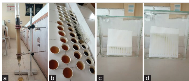
Figure 1: Column chromatography images. (a) Running column; (b) collected fractions; (c and d); thin-layer chromatography study of column fractions
