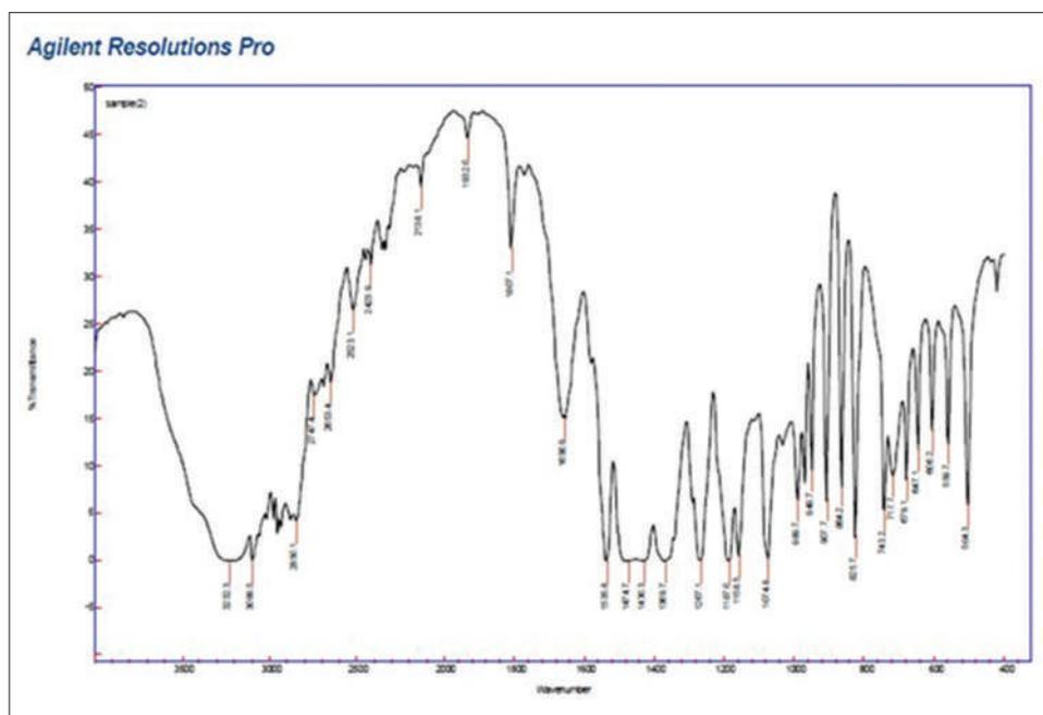
Figure 8: IR spectrum of metronidazole and its crud
